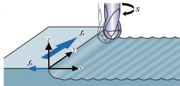
(b) Cutting Tool Movement Direction
