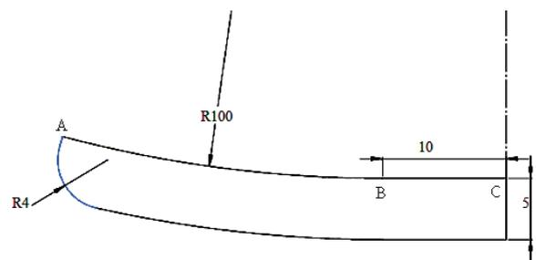
(c) Dimension of the die (Arc AB forms  $15^\circ$  angle at its center)
