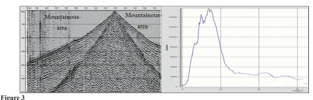
The Original Record and the Spectrum 3D Seismic in YSHS Field (Mountainous Area)
