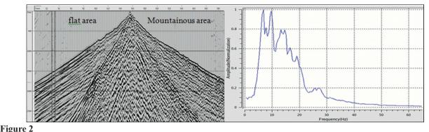
The Original Record and the Spectrum of 3D Seismic in DWS Field (Piedmont)
