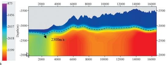
Figure 10 3D Seismic near Surface Tomography Model YSHS Field
