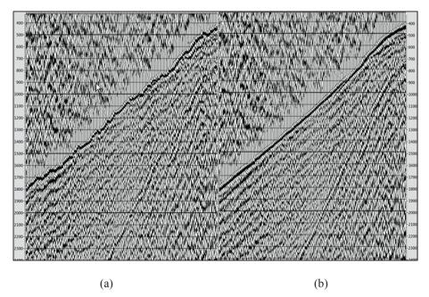
Figure 19 The Variation Characteristics of the First Break and the Interference Wave Before (a) and After (b) Static Correction
