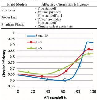
Figure 14 Circulation Efficiency with Sensitivity to ξ and Standoff
