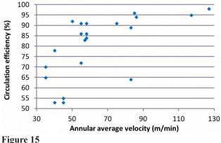
Effect of Annular Velocity on Circulation Efficiency
