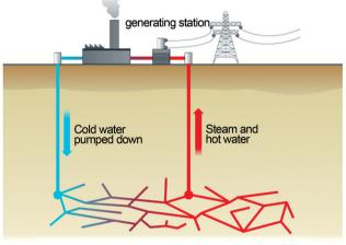
Figure 4 Geothermal Basic Principles
