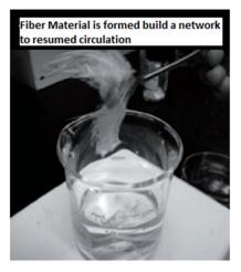
Figure 8 Cementing Loss Circulation Fiber Material's Ways of Working
