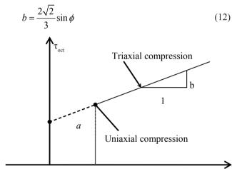
Figure 2 Mogi-Coulomb Failure Envelope
