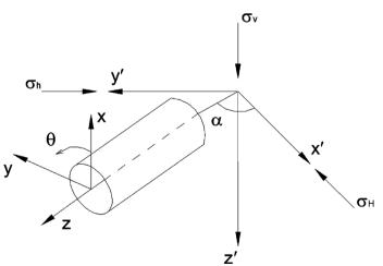
Figure 4 Stress Transformation System for a Horizontal Borehole
