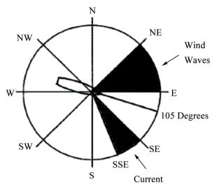
Preferred Rlg Heading:105 Degrees True Figure 8 Preferred Rig Heading Based on Rig Motions
