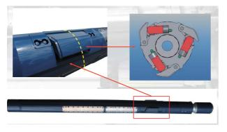
Figure 2 RSM Steering Blades Working
