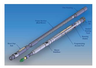
Figure 1 Component of RSM System
