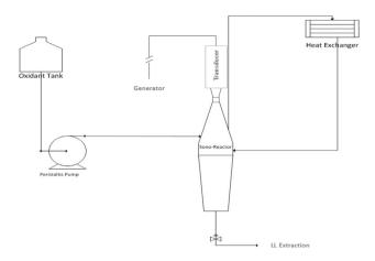
Figure 1 Schematic of Ultrasonic Assisted Oxidative Desulfurization Reactor
