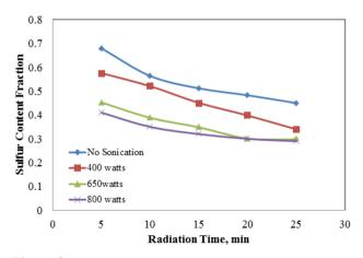
Figure 8 Role of Ultrasonic Wave Power on Percentage of Removed Sulfur
