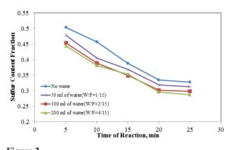
Figure 2 Role of Volume of Water Emulsified in 750 ml of Diesel on Desulfurization Process
