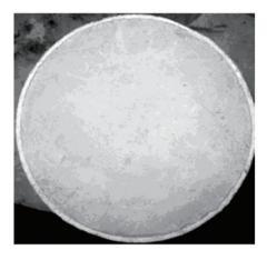
Figure 4 Set Cement Rock Sample
