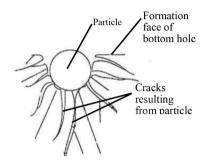
Figure 1 Sketch Map of Particle Impact Rock-Cutting Cracks
