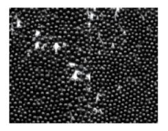
Figure 3 High-Carbon Cast Steel Shots
