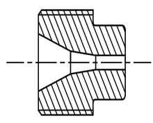
Figure 5 Double-Taper Nozzle
