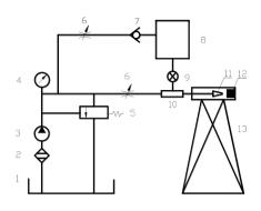
Figure 2 Schematic Diagram of Particle Water Jet Rock Breaking Experimental Setup
