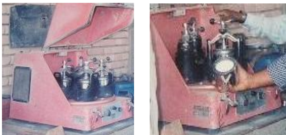
Fig. 4: Ball Mill for Grinding of Collected Samples to Very Fine Grain Size
