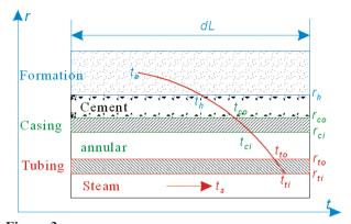
Figure 3 Schematic Diagram of Temperature Distribution During Steam Injection
