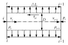
Figure 2 Micro-Unit of the Horizontal Wellbore
