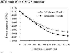
Figure 6 Steam Pressure Distribution Along Horizontal Wellbore
