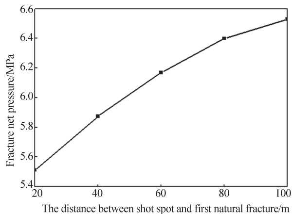
Figure 6 Relationship of Static Pressure At Fracture Opening and Location of Natural Fracture
