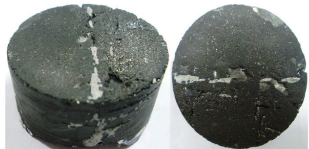
Figure 2 Shut Off Capacity of Bridging Type Preflush to No.3 Coal Seam Core of Qinshui Basin
