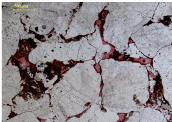
(a) S299 well, 3,456.20 m, intergranular pores-solution pores of I
