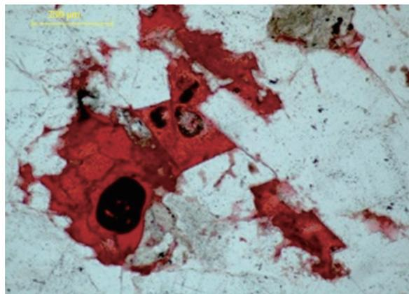
(b) S124 well, 3,628.32 m, dissolution pores of II
