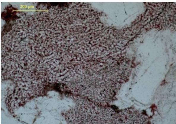
(c) S110 well, 3,736.42 m, alteration kaolinite intercrystalline pores of III
