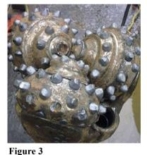
Bit Teeth Enlarge Figure After Construction Roller Bit After Construction
