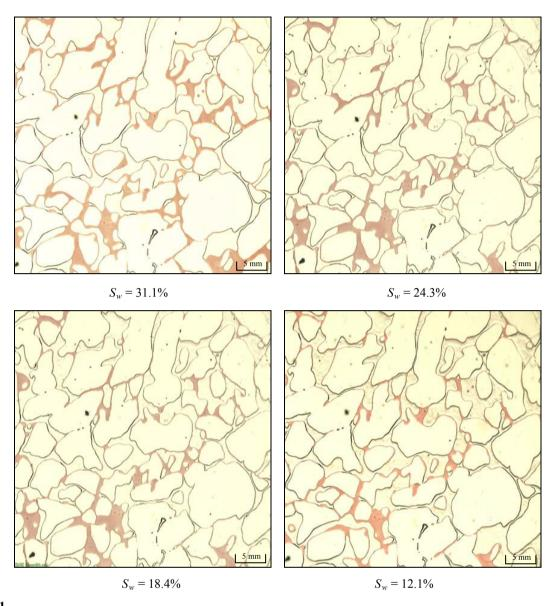
Figure 1 Distribution Characteristics of Gas-Water Saturation in the Process of Constant-Speed Gas Production Under a Pore Pressure of 0.5 MPa
