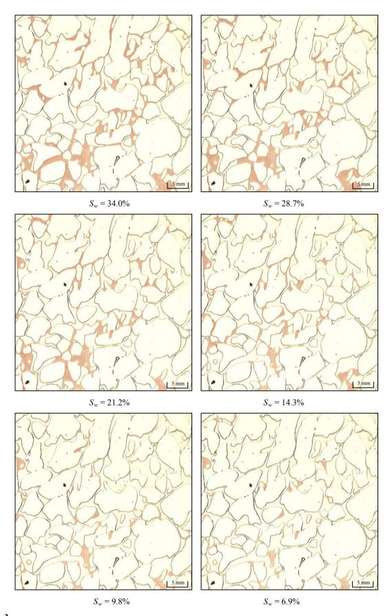
Figure 3 Distribution Characteristics of Gas-Water Saturation in the Process of Constant-Speed Gas Production Under a Pore Pressure of 5 MPa
