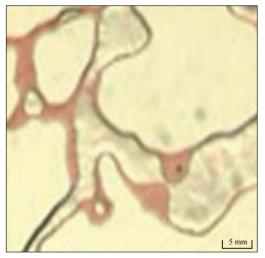
Figure 4 Microscopic Mechanism of the Seepage and the Distribution of Gas-Water During the Gas Production Process
