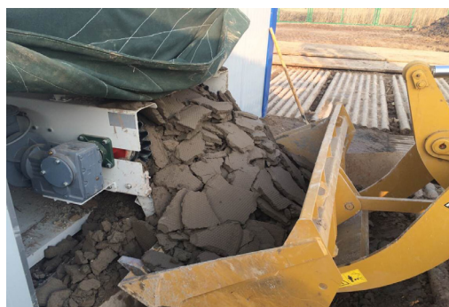
Figure 3 The Filter Pressing Process of Non-Landing Process for Drilling Fluid
