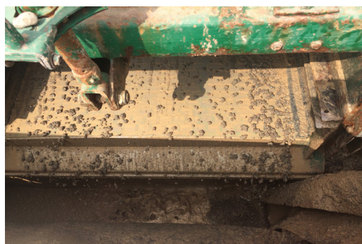
Figure 4 Sand Return of Compound Salt Drilling Fluid
