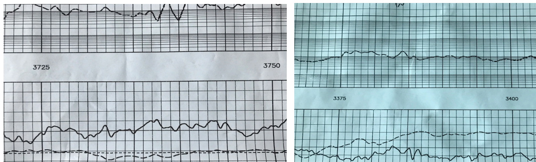
Figure 1 & 2 Logging Curve of Well Y22-x96 and Fx801 (the Dotted Line is Well Diameter)
