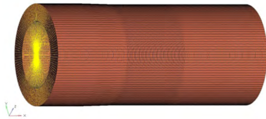
Figure 4 Finite Element Model of the Thickened Transition Section
