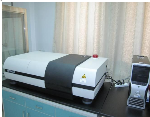
Figure 4: Sky scan 1172 high resolution CT
