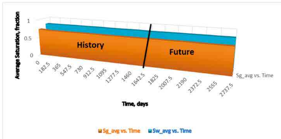
Figure C-16 Average Gas Saturation ( S_{g_{avg}} ) in Gas Invaded Zone and Average Water Saturation ( S_{w_{avg}} ) in Water Invaded Zone versus Time for the Egyptian Oil Field –Case (3)
