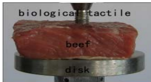
Fig. 1: The mechanical structure of testing beef pressure characteristic curves
