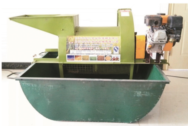
Figure 2 Photo of Threshing Separator and Control System
