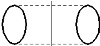
Figure 21 Toroidal Hull With Elliptical Cross Section at an Angle 0
